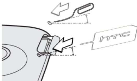
2. Pull the microSIM card tray out, and place the microSIM card into the tray.
